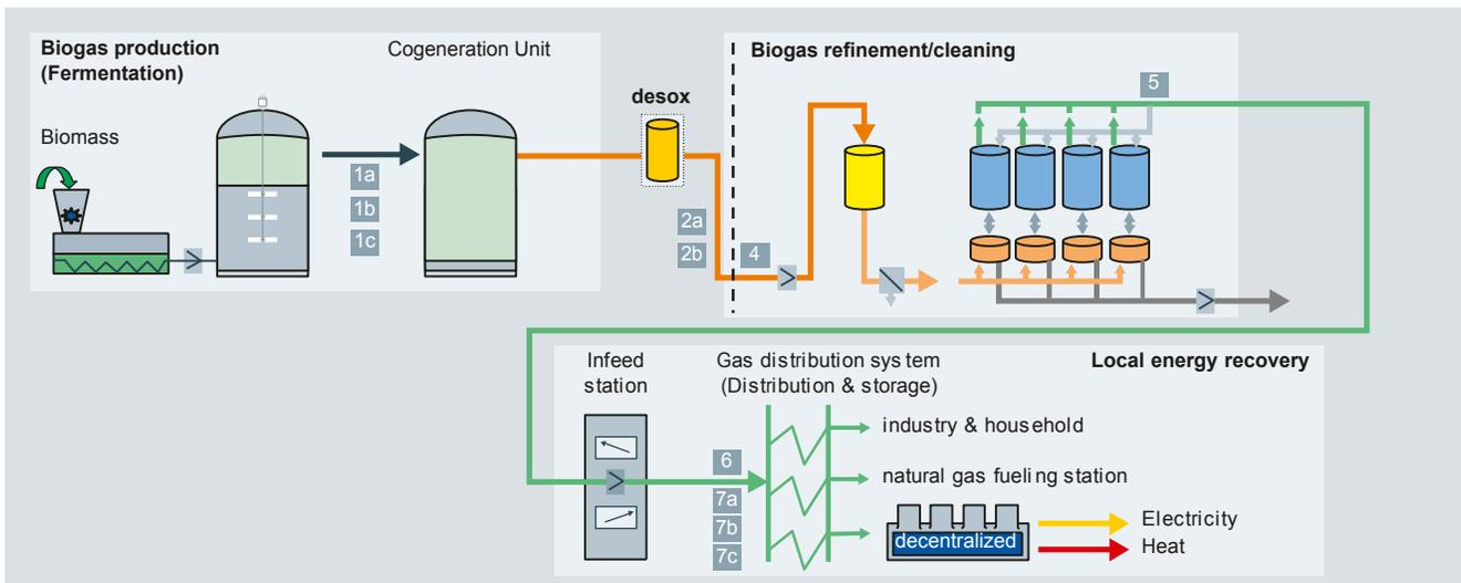
Fig. 2 Feeding of biomethane into the public gas network
